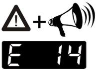
This safety installation is independent of the control circuit. When the temperature of the bath fluid has reached the safety temperature (85 °C), a complete shutdown of the compressor and pump is effected. The alarm is indicated by optical and audible signals (continuous tone) and on the LED-DISPLAY appears the error message "Error 14".
