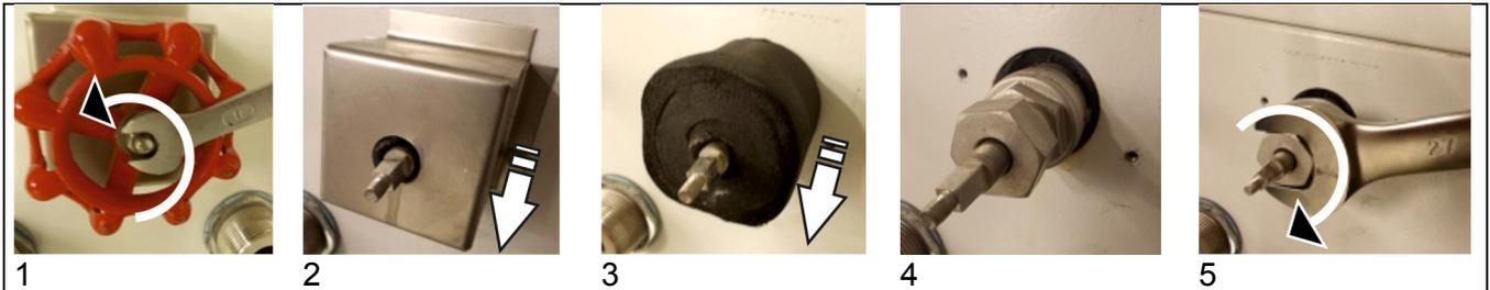
1. Undo the nut (a.f. 8) and remove the hand wheel on the adjustment valve,
