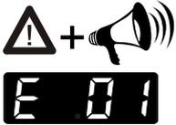
This safety installation is independent of the control circuit. If the low liquid level protection device is triggered, a complete shutdown of the compressor and circulating pump is effected. The alarm is indicated by optical and audible signals (continuous tone) and on the LED-DISPLAY appears the error message "Error 01".
