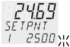
1. By pressing the key
