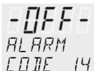
This excess temperature protection is independent of the control circuit. When activated heater and circulating pump are completely shut down. The alarm is indicated by optical and audible signals (continuous tone) and the error message "ALARM-CODE 14" appears on the VFD COMFORT-DISPLAY together with the ticker:
